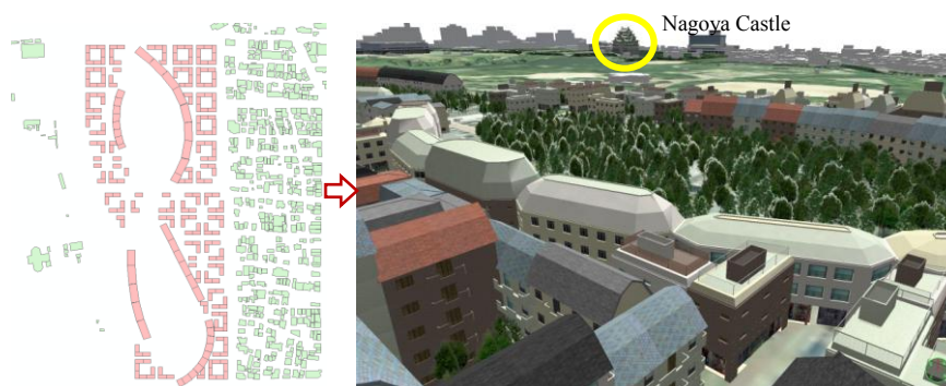
Fig.5. Proposed layout for the town and an automatically generated 3D urban model: terrace houses sharing green spaces in large courtyard, laid out for viewing Nagoya castle
